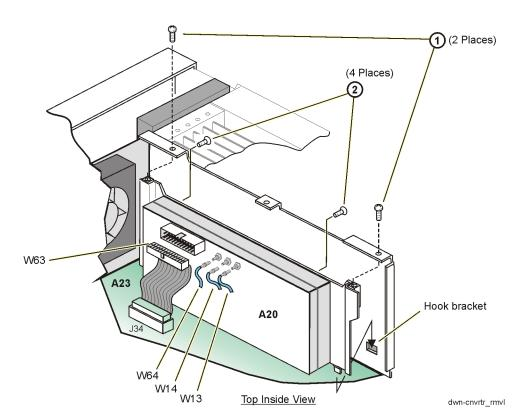
Figure 2-24 A20 Downconverter (Option 501, 502, 503, 504 with Option 300)
