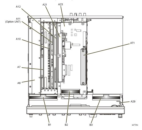
Figure 3-4 Assemblies from a Top View (Option 506)
