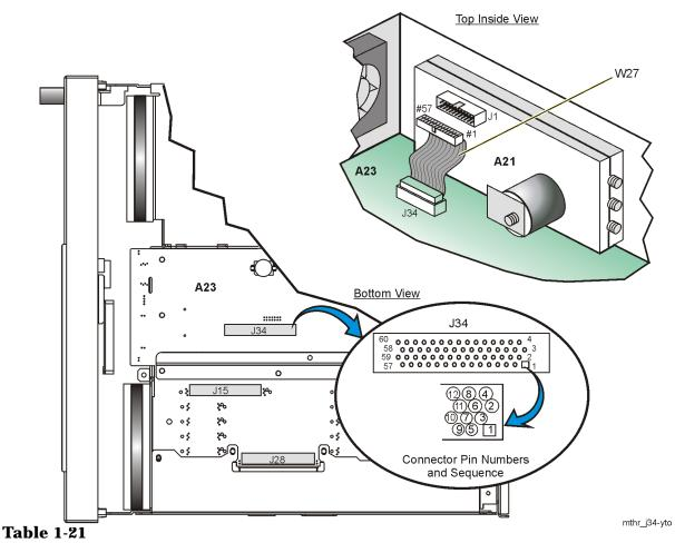
Power **Connector Pins on the** Minimum Maximum Origin **Supply** Value (Vdc) Value (Vdc) Voltage **A21 YTO Driver A23** (Vdc) (Option UNJ or **Motherboard** Option 506) +32 J1-55, 57 J34-55, 57 +31.04+32.96Main Supply J1-54, 56 J34-54, 56 +15 +14.1+15.9Main Supply J1-49 J34-49 -14.1-15-15.9Main Supply J34-50 -5.356-5.2J1-50 -5.044Main Supply J34-51 +5.72+5.2J1-51 +4.68**Main Supply** +5.2 VD J1-44 J34-44 +4.68+5.72Main Supply +3.4 VDY J1-45 J34-45 +3.298+3.502Main Supply
