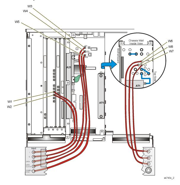
Figure 3-25 Option 506 - Front Panel Cables
