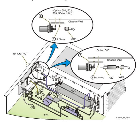
Figure 2-41 RF Output Connector for Option 1EM
