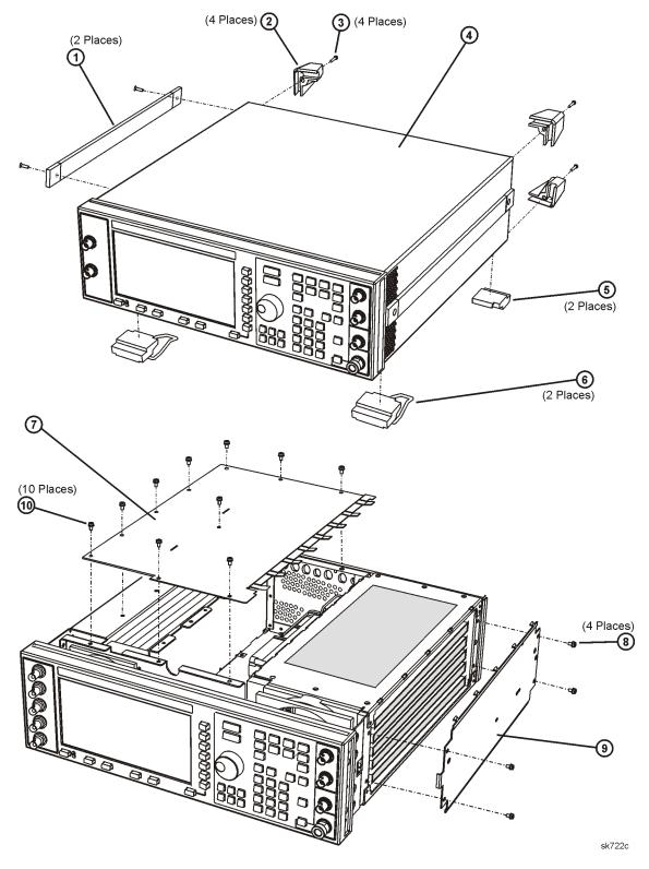
Figure 2-1 Outer and Inner Instrument Cover Removal
