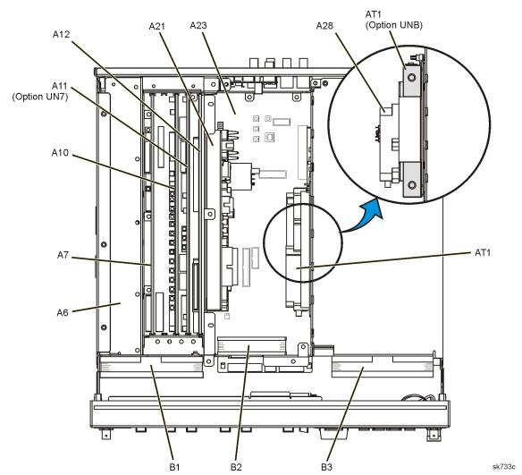
Figure 3-3 Assemblies from a Top View (Option UNJ)
