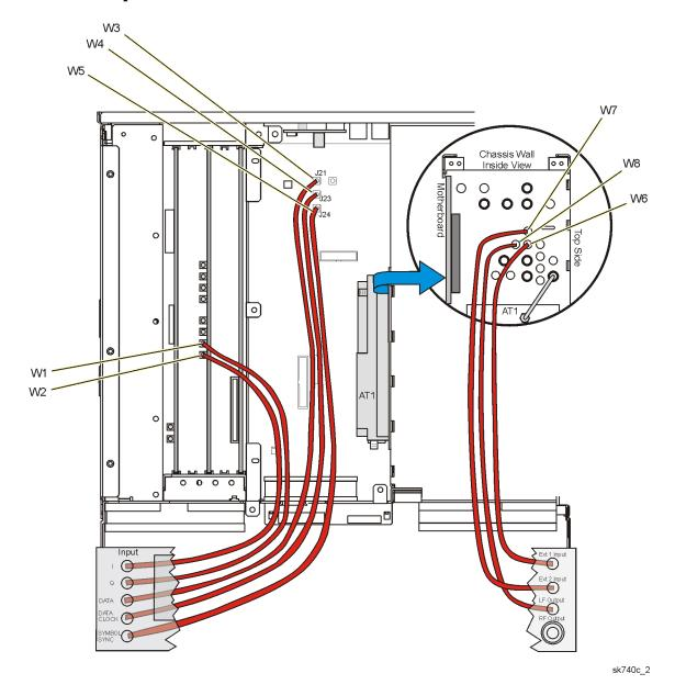
Figure 3-11 Option 501, 502, 503, 504 - Front Panel Cables
